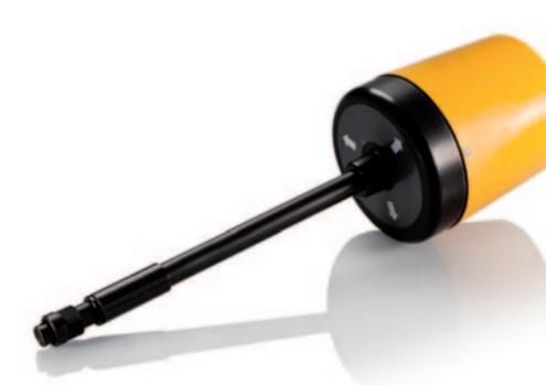
**E field probe Type EA/EB/EC/ED 5091**
